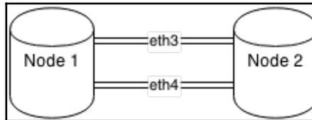
In some cases, it can be advantageous to connect the database servers to a general network fabric. Depending on the interaction of the upstream network devices, this can significantly increase the network packet's **round-trip-time (RTT)**. This is usually fine for PostgreSQL replication, but OLTP systems may be more sensitive. Block-level replication systems, such as DRBD, which operate beneath the filesystem, fare even worse.
