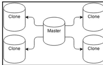
In this kind of model, the master node is tasked with transmitting transaction streams or WAL files to every node in the cluster. This makes it fantastically difficult to change the active master node and potentially overloads the master node itself. The primary write node of any cluster should be focused on fulfilling client requests. The purpose of `walctl` is to impose a structure like this:
