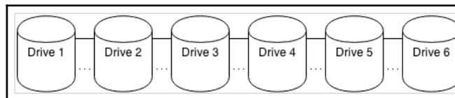
The solid line shows that the data is spread across all six drives. The dotted line is the parity information. If a drive fails and the block can't be read directly from the necessary location, a RAID 5 will use the remaining parity information from all drives to reconstruct the missing data. The only real difference between a RAID 5 and a RAID 6 is that a RAID 6 contains a second parity line, so up to two drives can fail before the array begins operating in a degraded manner.
