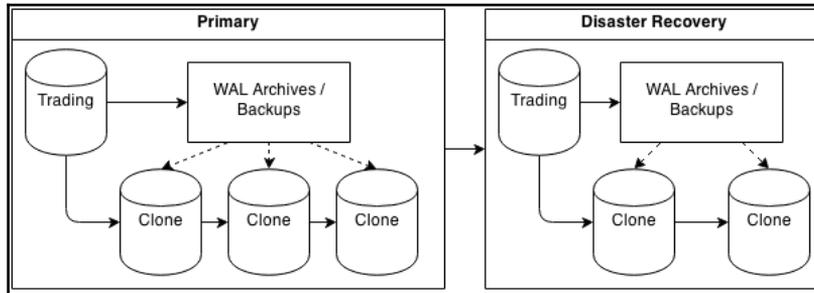
This diagram represents seven PostgreSQL servers for a single source of data. The Trading server sends its WAL data to a secondary system for safekeeping. One replica subscribes directly to the **Trading** database, while two others acquire their data through cascading replication. All clones are attached to the WAL archive in case their respective streams get disconnected.
