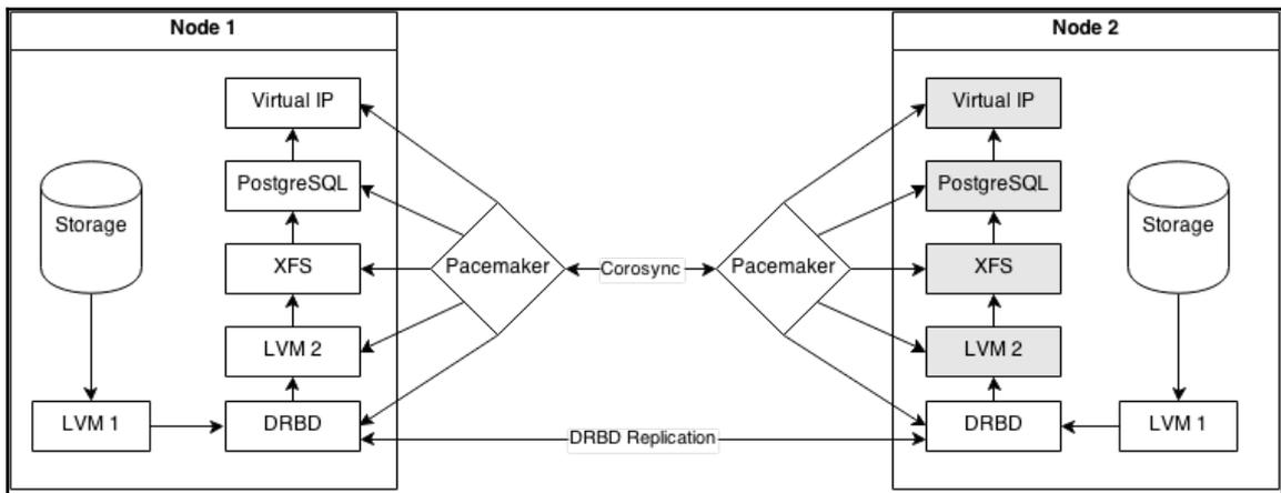
Here, all of the components are installed on both nodes, but the greyed-out ones are unavailable on **Node 2**. Yet, we could use Pacemaker to reverse the graph so that **Node 2** is the active server instead of **node 1**. That is a lot of changes to make manually.
