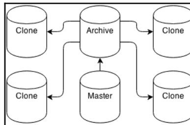
Instead of forcing the master node to supply each standby, the master transmits WAL data to a central archive server. Then, each clone can pull from that location as needed. In this recipe, we will install walctl so that we can take advantage of the structure it advocates.
