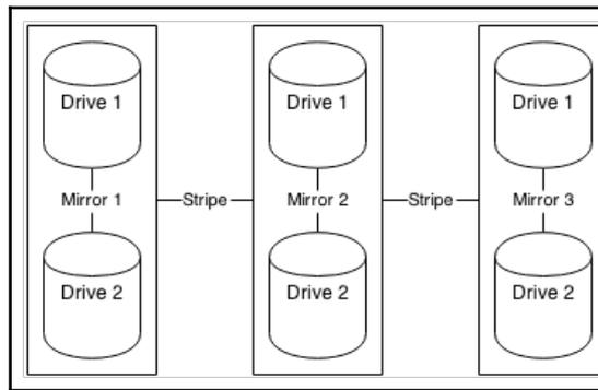
In this RAID 1+0, we have three sets, each consisting of two disks. Each of the two disks mirror each other, and the data is striped across all three sets. We could lose a disk from each set and still have all of our data. We only have a problem if we lose two disks from the same set, since they mirror each other. Overall, this is the most robust RAID level available, and the most commonly used for OLTP systems.
