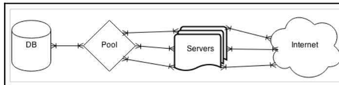
By inserting a connection pool in front of the database, hundreds of PostgreSQL server processes are reduced to dozens. A database pool works by recycling database connections as soon as the client completes its current transaction or when its database work is complete. Instead of hundreds of mostly idle database connections, we maintain a specific set of highly active connections.
