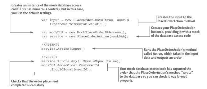
The mocked class, MockPlaceOrderDbAccess, doesn't access the database, but it has properties or methods that you can use to control every part of the reading of data from the database. This class also captures anything the PlaceOrderAction's method tries to write to the database, so you can check that too. This shows the mock database class, MockPlaceOrderDbAccess.
