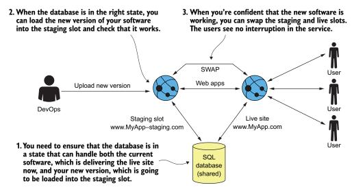
Figure 11.8 Azure provides a continuous service to the user when deploying a new version of the software. In Azure, you have a deployment slot, often called staging, where you can run up your new application ready to take the load. When you're happy with how it's working, you can swap the deployment slots, and your new code will take over. The important point from the EF Core/database perspective is that the database must be in a state that both your current and new software can use.
