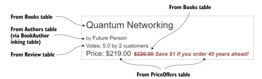
Figure 2.5 A listing of a single book showing which database table provides each part of the information
