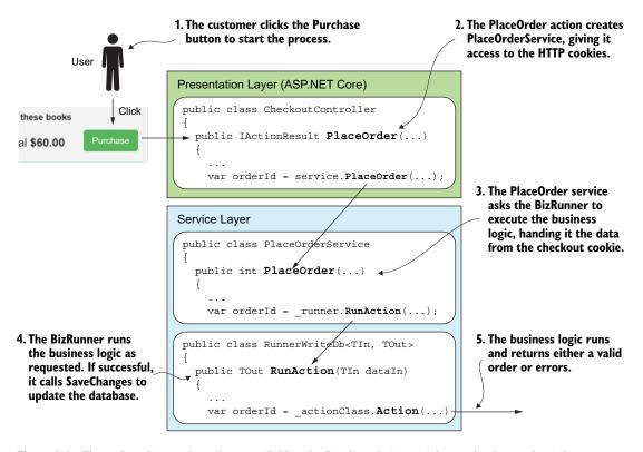
Figure 4.4 The series of steps, from the user clicking the Purchase button, to the service layer, where the BizRunner executes the business logic to process the order
