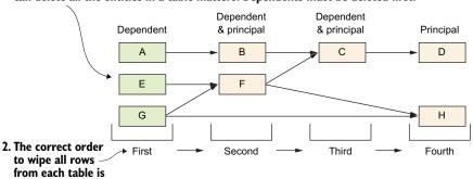
Figure 9.8 Each rectangle represents a table in the database that you want to delete all rows from. Because of the foreign-key links—which may have a cascade delete setting that precludes deleting a row because another row points to it with a foreign key—the order in which you delete rows from a table matters. The row at the bottom defines the correct order for deleting all the rows from a table.
