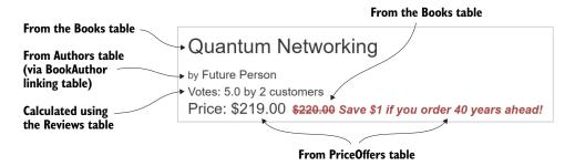
Figure 12.5 Select queries provide the best-performing database access, in which the final result consists of a mixture of columns from multiple tables.
