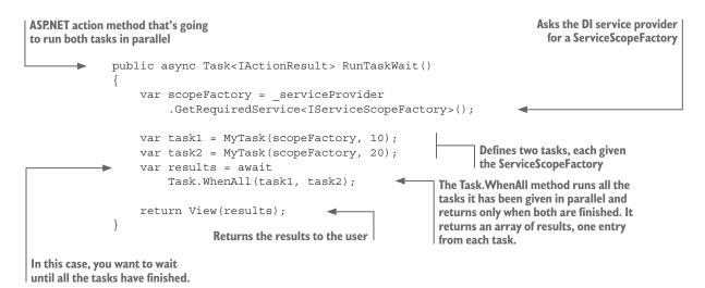
The important point from the code is that you provide ServiceScopeFactory to each task, so that it can use DI to get an instance of the DbContext (and any other service that has been registered).
