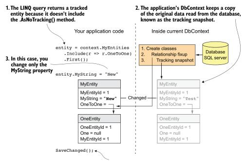
4. When SaveChanged is called, EF Core's DetectChanges method will run and compare an entity with a State of Unchanged with the tracking snapshot to see if anything is modified. It will also set the IsModified flag on those properties that are different.
