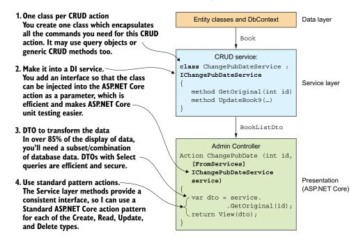
Figure 10.3 Four key patterns I've developed to speed up the writing of CRUD commands using the EF Core framework inside an ASP.NET Core application. Your pattern might be different, but developing your own pattern will make you quicker and less error-prone.
