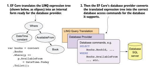
Figure A.1 Some book query code (bottom left) with its expression tree above it. EF Core takes the expression tree through two stages of translation before it ends up in the right form for the database that the application is targeting.
