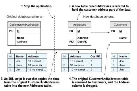
Figure 11.7 The steps in changing a database schema that requires data to be copied to ensure no loss of data. In this case, the application software is stopped while the database schema change is applied and data is copied to the new Addresses table. When that has finished, the new application software can start.
