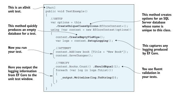
Figure 15.2 This gives you a flavor of some of the unit-test features covered in this chapter. Some of these methods are also available in a NuGet package called EfCore. Test Support.
