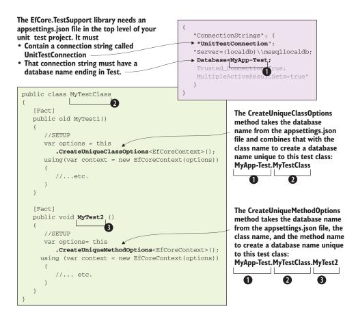
Figure 15.3 Two methods that set up the database options for an SQL Server database, but alter the database name to be either class-unique, or class-and-method-unique. When you run multiple unit test classes, they'll have their own databases, which means they won't interfere with each other.
