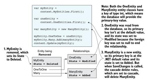
Figure 9.4 Updating an entity with both a Db generated key and not default value and a Not Db generated key, or key is default value relationship. The "Db generated key and not default value" case is shown in step 2. The "Not Db generated key, or key is default value" case is shown in step 3.
