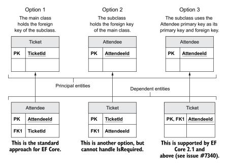
Figure 7.5 The three ways of defining a one-to-one relationship in a relational database; comments at the bottom indicate EF Core's handling of each approach. The difference between option 1 and option 2 (and 3) is that the order of the two ends of the one-to-one relationship are swapped, which changes which part can be forced to exist. In option 1, the Attendee must have a Ticket, whereas in options 2 and 3, the Ticket is optional for the Attendee.
