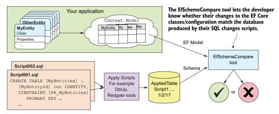
Figure 11.6 The EfschemaCompare tool compares EF Core's model of the database, which it forms by looking at the entity classes and the application's DbContext configuration, with the actual database schema. It will output human-readable error messages if it finds a difference.
