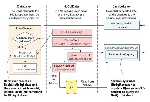
Figure 14.3 Internals of the NoSqlDataLayer are hidden from the DataLayer and ServiceLayer. The DataLayer and ServiceLayer work with the BookListNoSql class, which maps to the book list view, and several interfaces. The aim is to make it easy to add the CQRS read-side database with minimal impact on the existing application. It also allows you to change the read-side database server with minimal refactoring to the code outside the NoSqlDataLayer.
