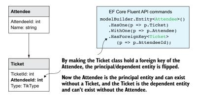
Figure 7.7 Option 2: The Ticket entity holds the foreign key of the Attendee entity. This changes which entity is the principal and dependent entity. In this case, the Attendee is now the principal entity, and the Ticket is the dependent entity.
