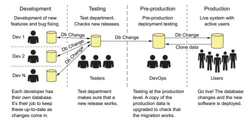
Figure 11.1 Various databases can be used in an application's development, all of which will need database schema changes applied to them. The terms development, testing, pre-production, and production refer to different parts of the development, testing, and deployment of an application and any associated database schema changes.
