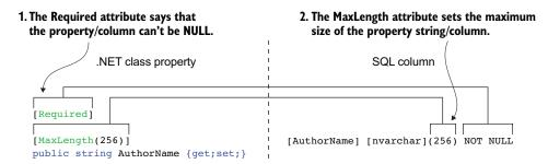
Figure 6.5 The [Required] and [MaxLength] attributes affect the mapping to a database column. The [Required] attribute indicates that the column shouldn't be null, and the [MaxLength] attribute sets the size of the nvarchar.
