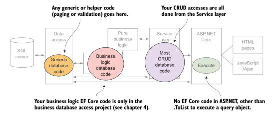
Figure 10.1 The application of the software design principle called separation of concerns to our layered architecture. Your EF Core code lives in two primary places: any database access that your business logic needs can be found in your BizDbAccess project, and the CRUD database accesses are all in the Service layer.
