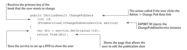
Line 3 in this listing is the important one. You've used parameter injection to inject, via DI, an instance of the ChangePubDateService class. The same line is also in the POST version of the ChangePubDate action.
