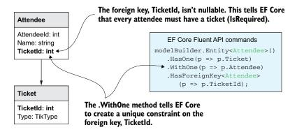
Figure 7.6 The non-nullable foreign key ensures that the principal entity (in this case, Attendee) must have a dependent, one-to-one entity, Ticket. Also, configuring the relationship as one-to-one ensures that each dependent entity, Ticket, is unique. Notice the Fluent API on the right has navigational properties going both ways—each entity has a navigational property going to the other.
