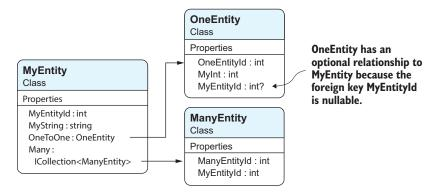
Figure 9.2 The examples that follow use these entity classes. OneEntity is an optional one-to-one relationship, because the foreign key back to MyEntity is nullable. OneEntity can exist in the database without being linked to MyEntity (its foreign key will be null). The ManyEntity entity class provides the Add command—creating a new entity/row in the database
