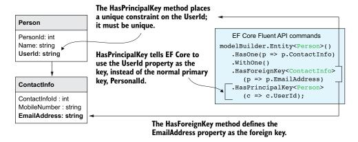
Figure 7.9 The Fluent API sets up a one-to-one relationship by using the UserId property, which contains the person's email address and is unique, as the foreign key to link to the ContactInfo. The command HasPrincipalKey both defines the UserId property as an alternate key and makes the foreign-key constraint link between the EmailAddress property in the ContactInfo entity and the UserId in the Person entity.
