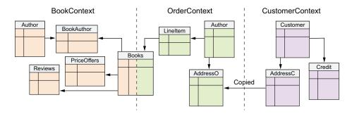
Figure 12.6 A large database can be split into multiple applications' DbContexts. In this case, the database is split along business lines. If you need to minimize application startup costs, you could create specific DbContexts for each application that contain only the entities that application needs to access.
