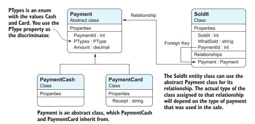
Figure 7.10 By using the Fluent API, you can create a more useful form of the TPH. Here an abstract class called Payment is used as the base, and this class can be used inside another entity class. The actual class type placed in the SoldIt payment property will be either PaymentCash or PaymentCard, depending on what was used when the SoldIt class was created.
