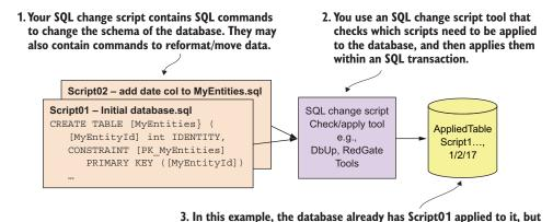
Figure 11.4 The process of applying SQL change scripts is normally handled by a tool that checks a table in the database to see what scripts have already been applied to the database. It then applies any missing scripts to the database.
