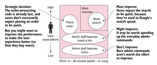
Figure 12.1 Various features from the book app graded with the user's expectations of speed on the vertical access, and the actual complexity/speed of the database access part of the feature. The type of user and user expectations have a big impact on what needs performance tuning.
