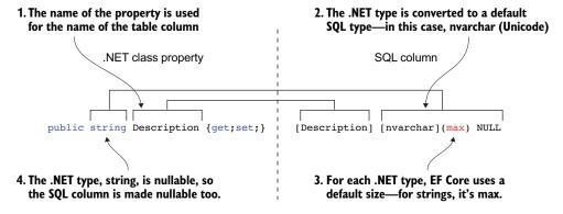
Figure 6.3 The application of the By Convention rules to define an SQL column. The type of the property is converted by the database provider to the equivalent SQL type, whereas the name of the property is used for the name of the column.
