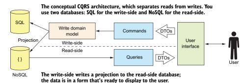
Figure 14.1 A conceptual view of a CQRS architecture with an SQL database for the write side, and a NoSQL database for the read side. A write takes a bit more work because it writes to two databases—the normal SQL database and the new NoSQL read-side database. In this arrangement, the read-side
