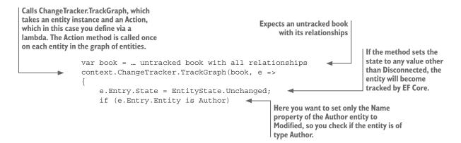
The result of running this code is that only the Author entity instance's State is set to Modified, whereas the State of all the other entity types is set to Unchanged. In addition, the IsModified flag is set only on the Author entity class's Name property.
