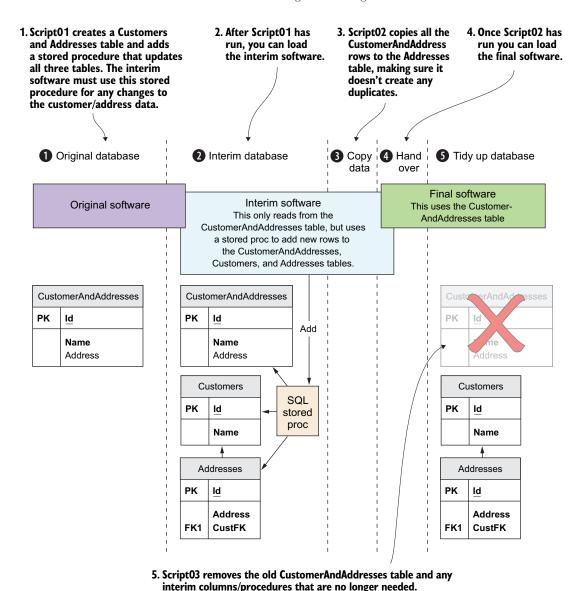
Figure 11.9 The five stages of changing a database when you want to supply a continuous service to your users. The three software versions—original, interim, and final—overlap to provide a continuous service. The interim software needs to read data from the original database structure because the original software is running in
