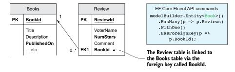
Figure 7.8 A one-to-many relationship, in which the foreign key must be in the dependent entity; in this case, the Review entity class. You can see in the Fluent API on the right that the Book has a collection navigational property, Reviews, linked to the Review entity classes, but Review doesn't have a navigational property back to Book.
