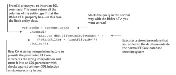
In the preceding code, you were querying an entity class property, which is all you could do up to EF Core 2.0. But from EF Core 2.1, you'll be able to use the FromSql method with a *query type*, which is a type that isn't an entity class (see appendix B, section B.1.5).
