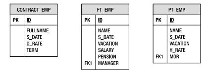
Figure 10-14. Table-per-concrete-class data model
