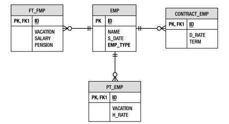
Figure 10-13. Joined inheritance data model
